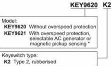
factory default setting is for AC generator sensing, calibrated to either 50 or 60 Hz nominal. Non-standard (NS) settings/options are available to order.
