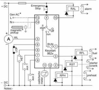
Overspeed models 9621 only. Select generator AC or magnetic pickup speed sensing using links J2 & J3 (see rear view diagram). Factory default setting is for generator AC sensing.
